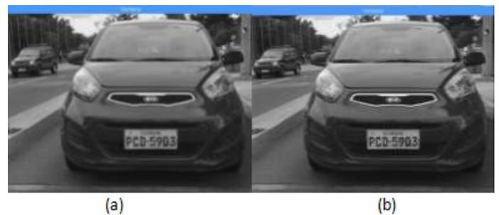
**Figure 5.** Gauss filter. (A) Mask 3x3. (B) 9x9 mask.
