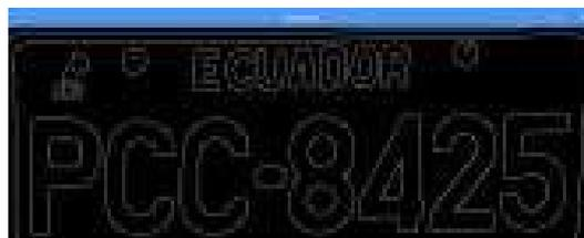
**Figure 13.** Edges of the vehicle plate.
