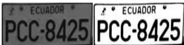
**Figure 11.** Binarization by the Otsu Algorithm.
