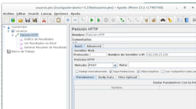
**Figure 3.** HTTP in Apache-Jmeter Requests Configuration.
