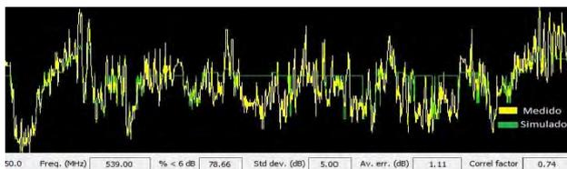
**Figure 9.** Correlation between propagation model ITU-R P.1546 without diffraction and field measurements.
