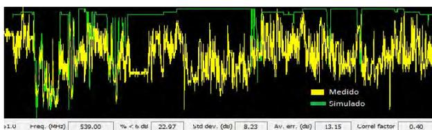
**Figure 10.** Correlation between ITU-R propagation model P.525 with Deygout94 diffraction and field measurements.
