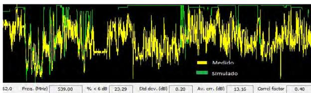
**Figure 11.** Correlation between propagation model ITU-R P.525/526 with diffraction Shape Rounded and field measurements.
