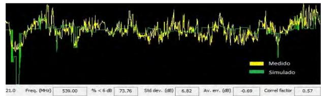
**Figure 7.** Correlation between propagation model ITU-R P.525 with diffraction Shape Rounded and field measurements.
