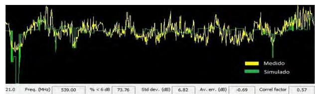
**Figure 8.** Correlation between propagation model ITU-R P.525/526 with diffraction Shape Rounded and field measurements.
