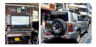
**Figure 2.** Station SACER sct-l01, with which the acquisition was made of samples in the cities of Ambato and Latacunga.
